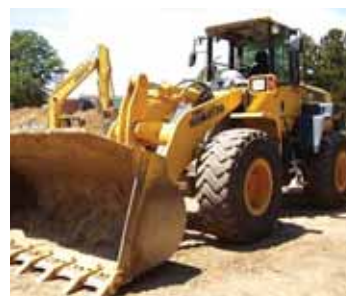
2011 Komatsu WA320-6 S/N C008686, 3,602 hrs., ROPS, enclosed cab, AC, limited slip diffs, ECSS ride control, addi- tional cwt., stereo, GP bucket with teeth, Turbo II pre-cleaner, Michelin radials, equipped with KOMTRAX, $138,000
