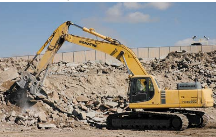
An Oxford Recycling operator uses a Komatsu PC300LC excavator with a pulverizer attachment to break up concrete.
