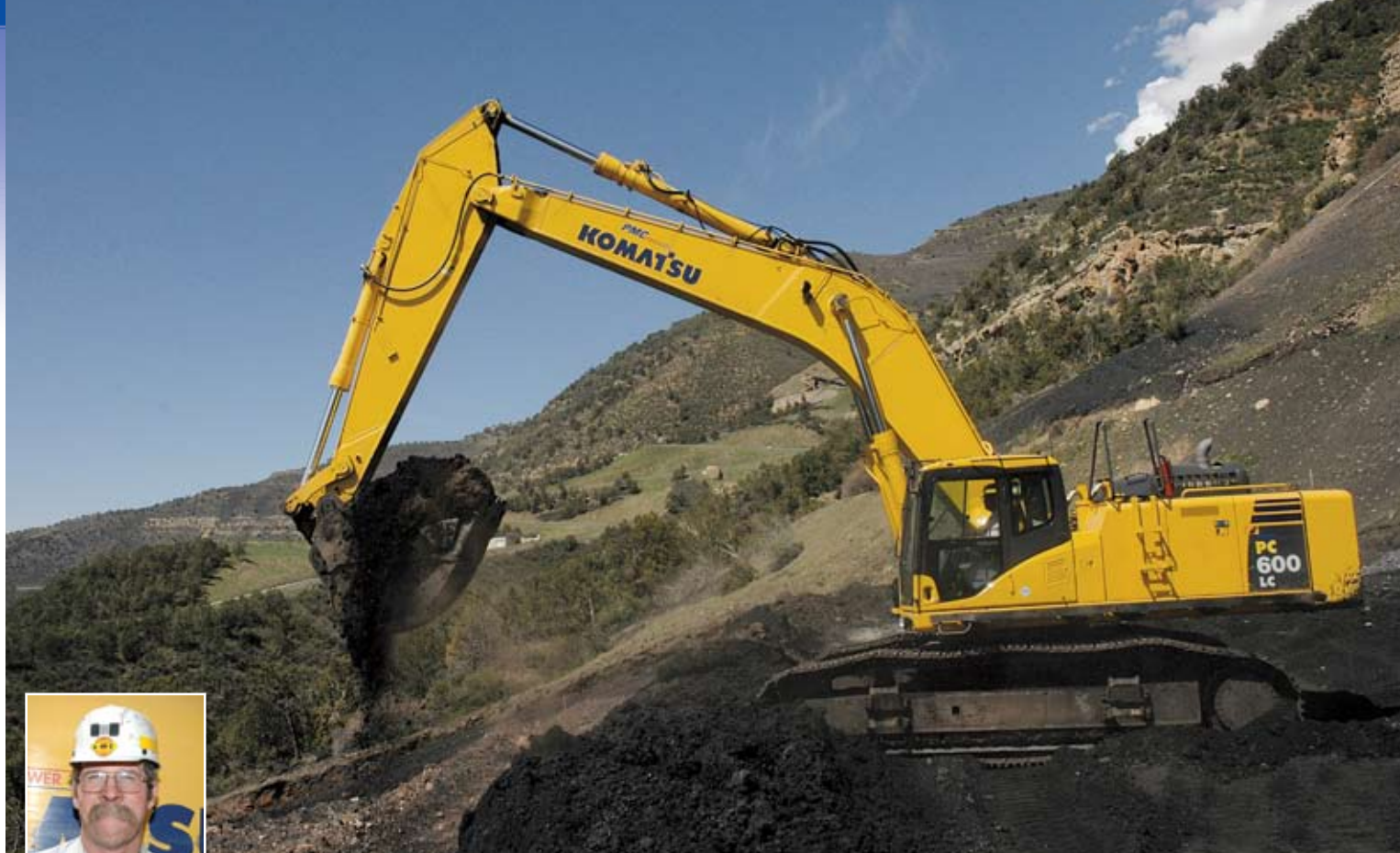
Operator Steve Kellerher uses a Komatsu PC600LC-7 to work the slopes on the refuse pile. "It's a workhorse," Kellerher said of the 133,000-pound excavator. "I can reach out and grab whatever I want and pull it out of the ground. It's a very good machine."
