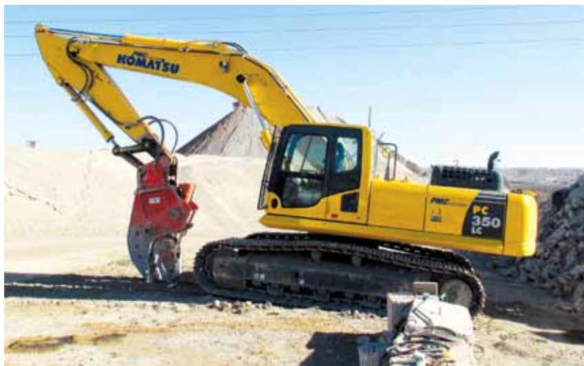
Oxford Recycling uses this Komatsu PC350LC-8 excavator, equipped with an NPK crusher, to pre-size concrete.
