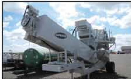
2006 Cedar Rapids Portable Wash Plant C006889: 4' x 10' 2 deck, Superior Single screw.....$58,000
