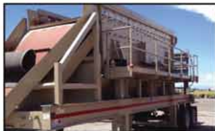
1999 KPI-JCI 6203 C006879: reconditioned, 6x20 triple deck portable screen, new switchgear, $105,000
