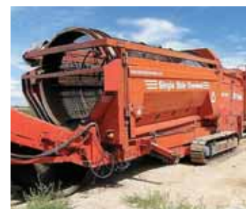
Finlay 770 S/N C006028, 3,481 hrs., 100 hp, 6'7"x17'1" Trommel Screen, Duetz 100 hp water-cooled diesel engine, 7.45-cu.-yd. low-profile hopper, 2.5" screen
