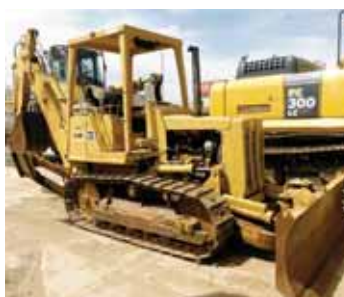
Caterpillar D3B S/N C009203, OROPS, PAT blade, rear backhoe
