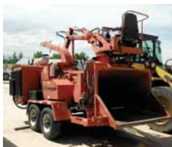
Morbark Woodhog S/N C009423, 515 hrs., self- contained 2400 XL Hurricane, 18" FEED, twin-disk clutch, self- feeding grapple
