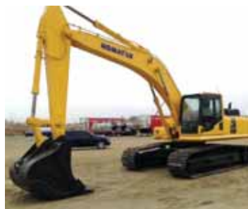
2011 Komatsu PC350LC-8 S/N C008534, AC, 10'7" arm, pattern-change valve, 60" bucket, equipped with KOMTRAX
