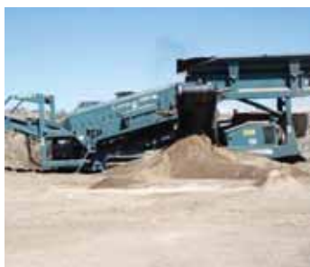
2004 Powerscreen Warrior 1800 S/N C006145, 8,826 hrs., Power Screen Warrior incline belt feeder with hydraulic hopper sides, folding conveyor, two-deck screen
