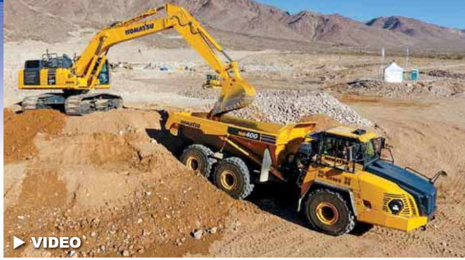
A Komatsu PC490LCi – the world's largest intelligent Machine Control excavator – loads an HM400 articulated haul truck at Komatsu's Demo Days in Las Vegas.
