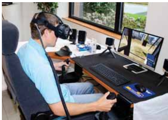
Using Komatsu's Worksite VR operator-training simulator, this customer completes a series of tasks on a computer-generated excavator.
