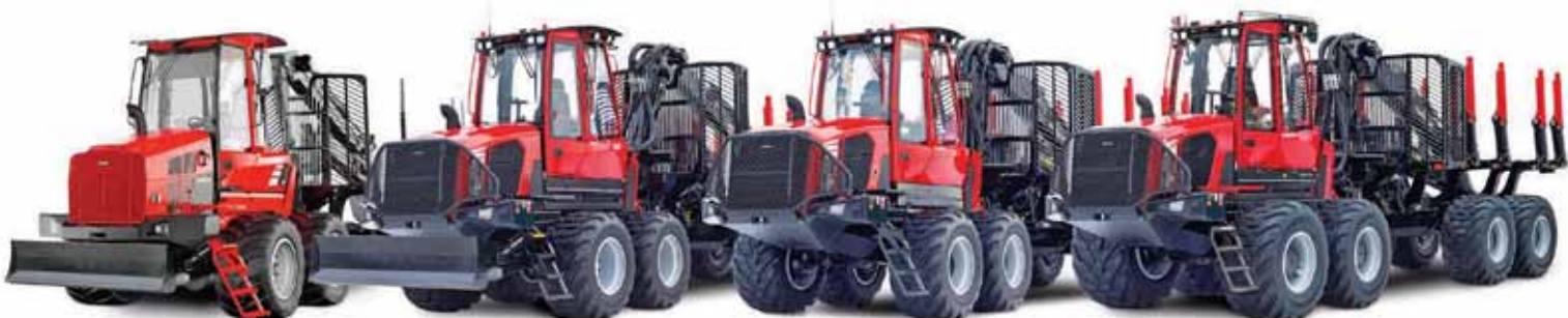
The new Komatsu 845, 855, 875 and 895 Tier 4 Final forwarders have rated payload capacities of 12, 14, 16 and 20 metric tons, respectively.
