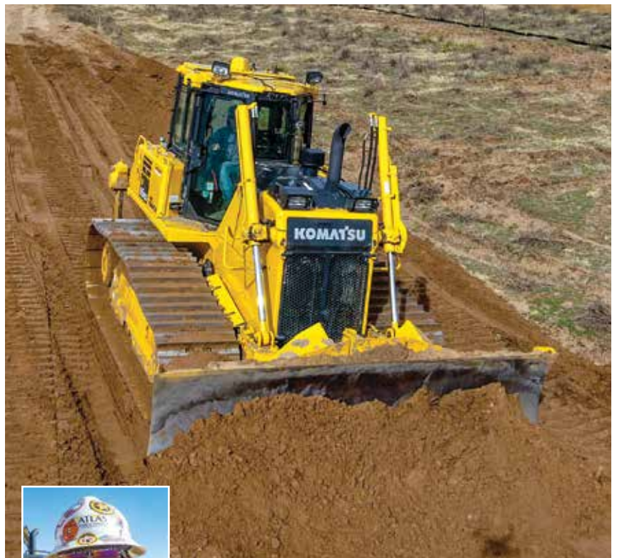
Gusher Oilfield Services Operator Casey Cook builds a well pad with an intelligent Machine Control Komatsu D65PXi-24, featuring integrated GPS grade control. “I like that there are no masts and cables to deal with or get in the way of visibility,” said Cook.
